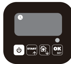
SLEEP PAGE: Landroid® is fully charged and is not in the working hours.
